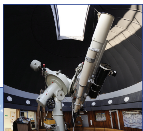
„South dome“ - telescope Newton 254/1200 + CCD G2 402 (Moravian Instruments)
