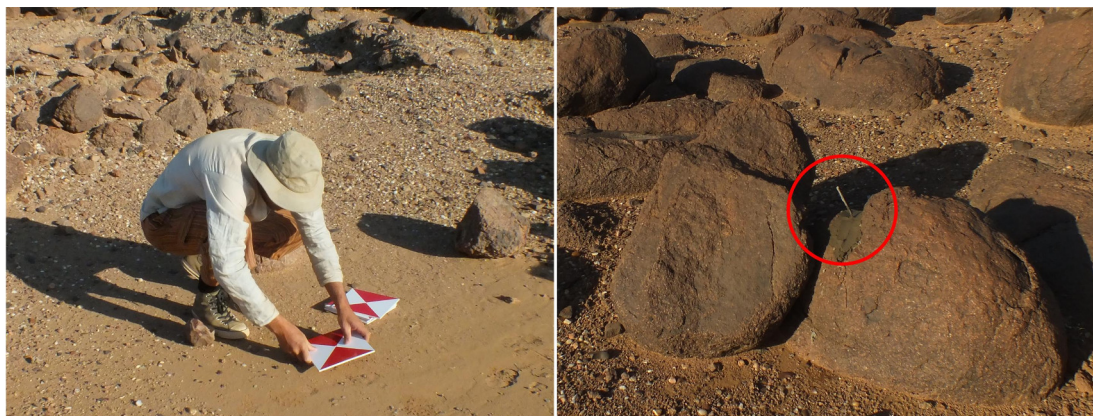
Figure 3: Points used as ground control points in the KAP survey (left), discrete fixed points (right).
