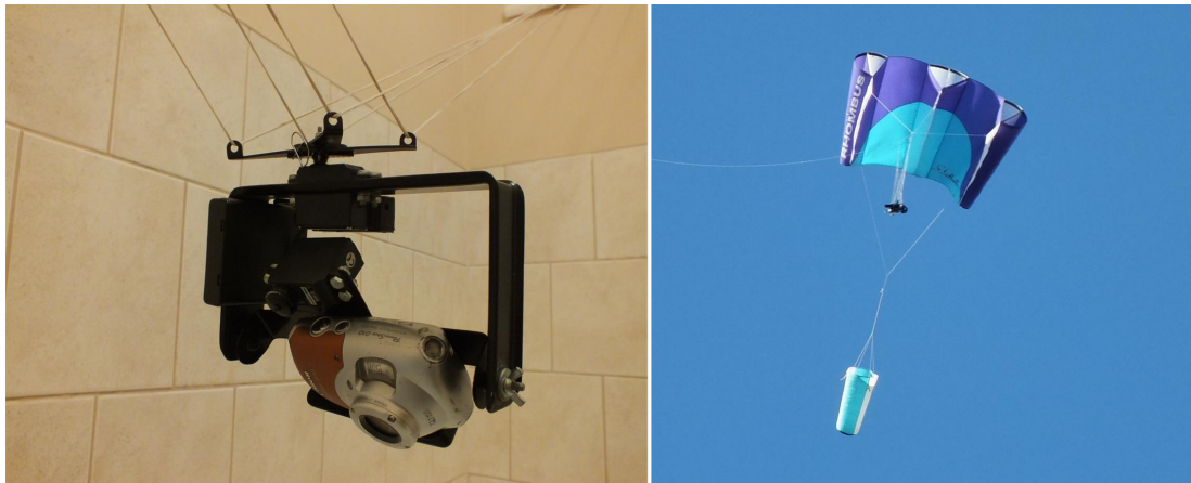
Figure 6: The Picavet suspension used on the Rhombus kite.
