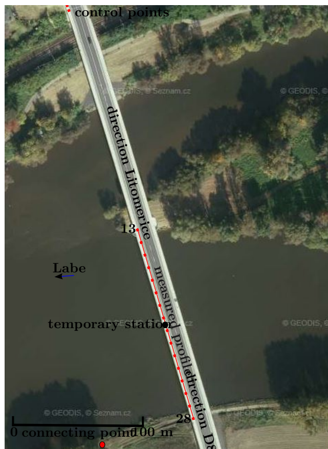
Figure 5: Configuration of measurement (Areal Image © Geodis)
