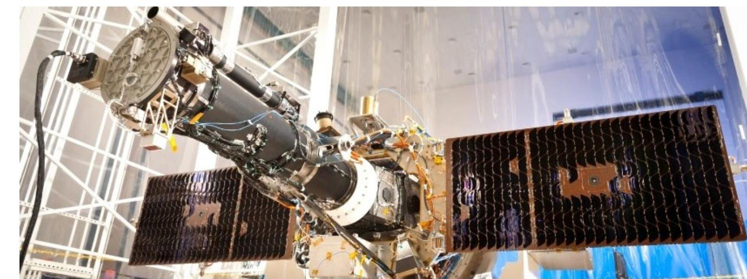
Atmospheric Imaging Assembly (**AIA**) on board Solar Dynamics Observatory (**SDO**)
