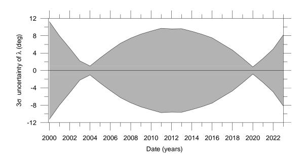
Fig. 9. Evolution of the 3- $\sigma$  uncertainty of the ecliptic longitude ( $\lambda$ ) of the radius vector of Dimorphos with respect to Didymos in time.
