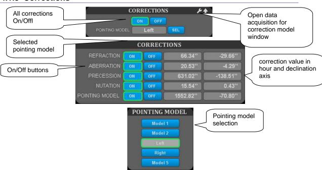
Any correction is possible to turn on/off by the appropriate button. The calculated value is displayed for both axis.
