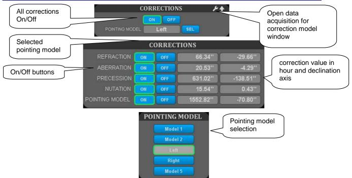
Any correction is possible to turn on/off by the appropriate button. The calculated value is displayed for both axis.
