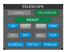
Check or update the DUT1 value in parameters 1 screen. Source of this value is in IERS BULLETIN - A, for example here: http://maia.usno.navy.mil/ser7/ser7.dat, section COMBINED EARTH ORIENTATION PARAMETERS, column UT1-UTC, value from the most recent date. The value can be also negative. Check also data acquisition parameters (on the parameters 3 screen) for fast centering of the star.
